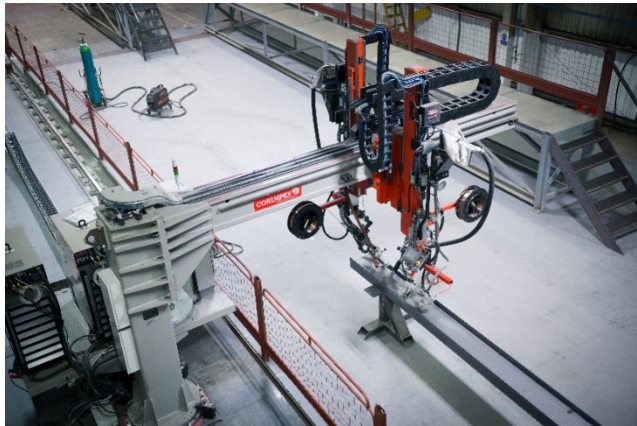
Corimpex Beam Welding Line
